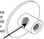
Cut chamfer here, both sides of tube
