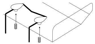
Carefully measure the wing wire distance and mark the same distance on the wing, centering the marks. Then cut two 7/32" holes for the wing mounts. Push the mounts into the wing, then push the wire through the mounts. Screw the set screws into the mounts from the bottom of the wing.
