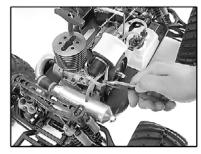
Always stop the engine before you turn the radio switches off. You can stop the engine by pinching the fuel line leading to the carburetor. Do NOT try to stop the engine by plugging the exhaust outlet or by stopping the flywheel with your finger or thumb.
