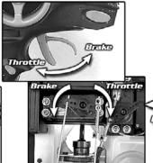
Pulling the trigger should open the carburetor throat, pushing the trigger should apply the brakes.
