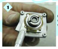
Check the gasket for signs of wear or breakage. Lift it away with your hobby knife carefully.
