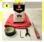
Before starting, assemble the following: 3m 3-in-1 brand or other lightweight oil, a small flat head screwdriver, your Allen wrench set, your wheel nut wrench, a roll of electricians tape, an old rag for wiping oil. Also have a hobby knife and needle nose pliers handy (not shown).
