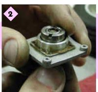
Push the starting axle back in all the way. Holding the parts as shown, rotate the bearing counterclockwise with your left forefinger and the axle head clockwise with your other hand from underneath to lubricate it thoroughly.
