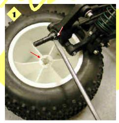
Put the wheel back on the axle, lining up the notches in the wheel with the pin on the axle.
