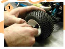
Use your wheel nut wrench to remove the nut from the rear wheel next to the engine.
