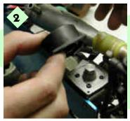
Transfer the cover to the other hand so your right forefinger holds the spring in place. Slip the pull start handle into position with your left hand and move the pull start into place over mounting holes.
