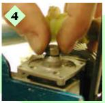
Rotate the axle head so the bearing notch seats in the crank shaft pin.
