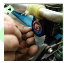
Bolt the pull start cover to the engine with the remaining four screws.
