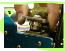
Remove the back plate from the engine. Your back plate may look slightly different.
